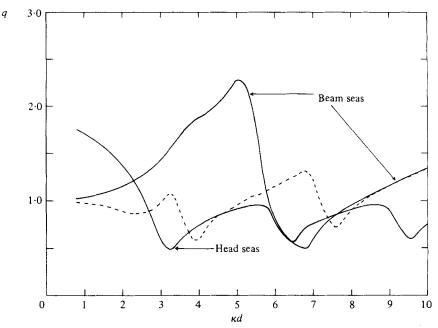
FIGURE 2. Variation of the mean gain factor q with the non-dimensional body spacing  $\kappa d$  for an optimally tuned single row of five equally spaced semi-immersed spheres for different values of the angle of incidence  $\beta$ . ——,  $\beta = 0$  (beam seas),  $\frac{1}{2}\pi$  (head seas); – – –,  $\beta = \frac{1}{4}\pi$ .
