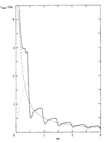
FIGURE 10. Variation of the non-dimensional maximum absorption length  $l_{max}/10a$  with frequency  $\kappa a$  for an optimally tuned row of five equally spaced semi-immersed spheres in beam seas. The spacing between the bodies is fixed at  $d = 12 \cdot 5a$ . ----,  $l_{max}/10a$  for unconstrained optimal motion; ...,  $l_{abs}/10a$  for constrained motion, maximum body displacement < three times incident wave amplitude; - - -, mean gain factor q = 1.
