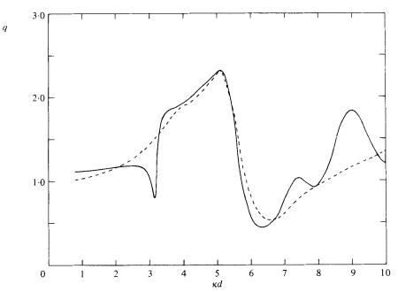
FIGURE 7. Variation of the mean gain factor q with body spacing for an optimally tuned double row and an optimally tuned single row of semi-immersed spheres in beam seas. The spacing between the rows of the double row is equal to the spacing between adjacent members of each row, i.e. c = d. ——, double row; – –, single row.
