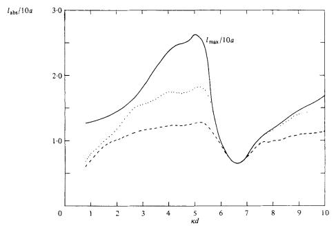
FIGIRE 6. Variation of the non-dimensional absorption length  $l_{abs}/10a$  with body spacing for the single row of semi-immersed spheres in beam seas. —, optimal unconstrained motion; ..., constrained motion, maximum body displacement < three times incident wave amplitude; - - - constrained motion, maximum body displacement < twice incident wave amplitude.
