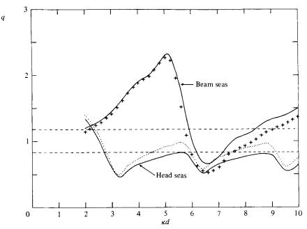
FIGURE 13. Variation of the mean gain factor q with non-dimensional body spacing  $\kappa d$  for an optimally tuned, single row of five uniformly spaced thin ships in beam and head seas. + + + (.....), the corresponding curves from figure 2 for five semi-immersed spheres in beam (head) seas. - -, the values corresponding to  $q_t = 1$  in beam (the upper line) and head seas.
