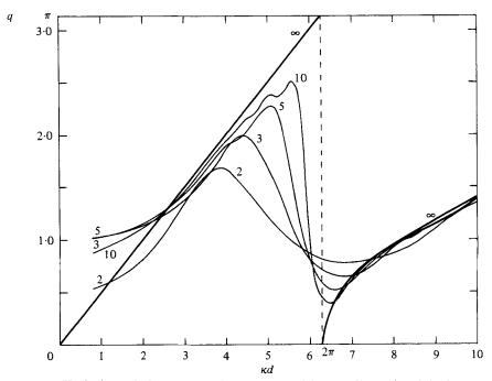
FIGURE 15. Variation of the mean gain factor q with non-dimensional body spacing  $\kappa d$  for optimally tuned equally spaced single rows of two, three, five and ten point absorbers in beam seas. The heavy solid line corresponds to the infinite array limit given for  $\kappa d < 2\pi$  by Evans (1979) and for general  $\kappa d$  by Srokosz (1980).
