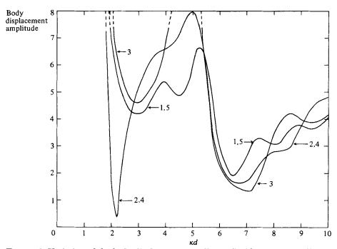
FIGURE 3. Variation of the body displacement amplitudes/incident wave amplitude with body spacing for the optimally tuned single row of five semi-immersed spheres in beam seas. The number next to each curve denotes the appropriate body motion.
