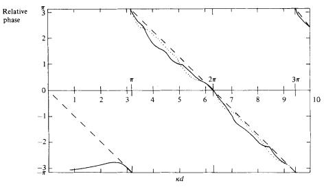
FIGURE 5. Variation of the relative phase, i.e. the phase difference between two adjacent bodies, with the body spacing for the optimally tuned single row of semi-immersed spheres in head seas. —, the relative phase of the (first and second) and (fourth and fifth) bodies; ..., the (second and third) and (third and fourth) bodies; ..., a constant phase difference of  $-\kappa d$ .
