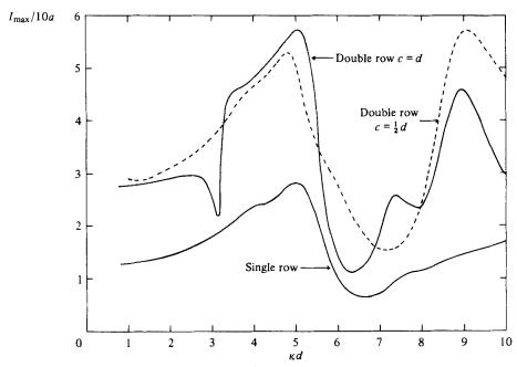
FIGURE 8. Variation of the non-dimensional maximum absorption length  $l_{max}/10a$  with body spacing for optimally tuned single and double rows of semi-immersed spheres in beam seas. The double row spacings are c = d and  $c = \frac{1}{2}d$  (indicated by a broken line).
