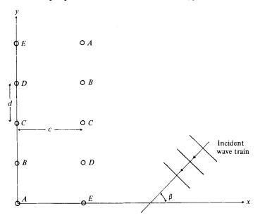
FIGURE 1. Plan of double-row array subject to incident wave train with arbitrary angle of incidence  $\beta$ . Bodies indicated by the same letter undergo the same displacement amplitude at optimal tuning. For the special cases of head and beam seas B = D and A = E (symmetry text given in § 3b).
