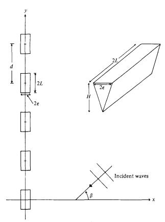
FIGURE 12. Diagrammatic sketch of thin ship and plan of five uniformly spaced thin ships in a single row.
