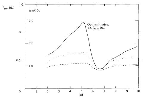
FIGURE 14. Variation of the non-dimensional absorption length  $l_{abs}/10L$  with body spacing for the single row of five thin ships in beam seas. ——, optimal unconstrained motion (i.e.  $l_{max}/10L$ ); ..., constrained motion, maximum body displacement < three times incident wave amplitude; – –, constrained motion, maximum body displacement < twice incident wave amplitude. The scale  $l_{abs}/10a$  is also shown to enable comparison with figure 6.
